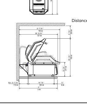
Plug In SpeeDelight with flexible top plate, flat, removable teflon plate
